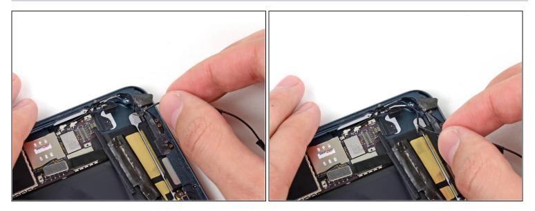
Pull the antenna cable away from its recess in the rear case.
