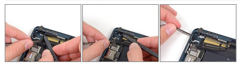
• Use the tip of a spudger to remove the small piece of tape securing the antenna cable in the bottom right corner of the iPad.
