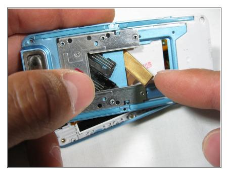
Slide ribbon cable through the slider mechanism.
