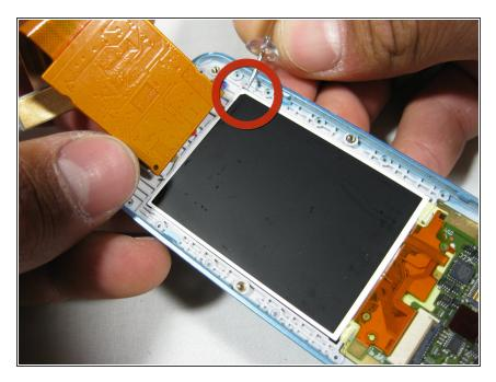
Lift the top edge of the screen using a pin to pry under the corner.
