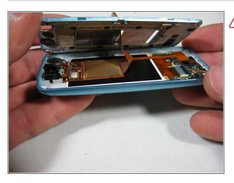
Carefully lift the slider mechanism to see the ribbon cables underneath.
