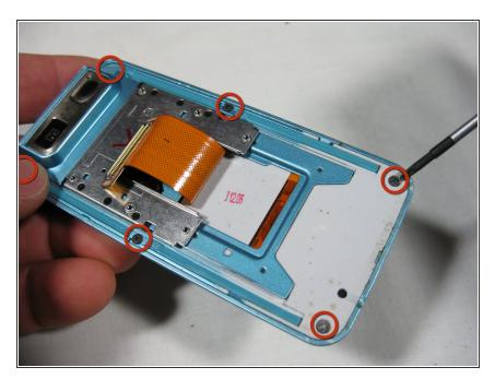
Remove the 6 screws with a Phillips #00 Screwdriver.
