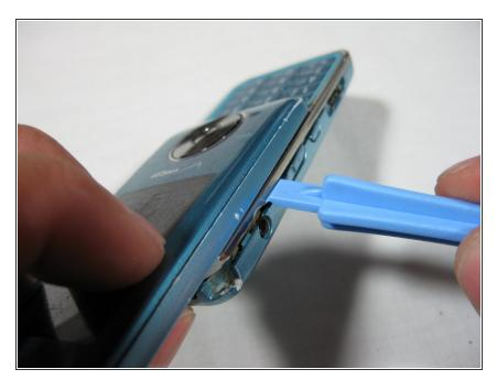
Use the iPod opening tool to pry off the back casing.
