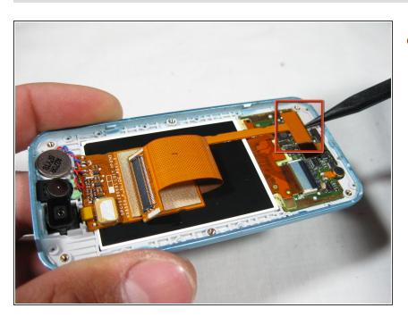
With the spudger, lift up under the connector to unplug it from the circuit board.
