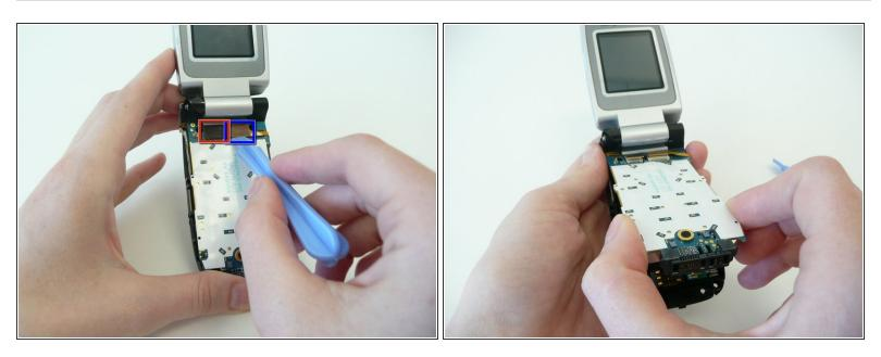
• Use the opening tool to remove the 2 ribbon wires (boxed in the photo) from the logic board.
