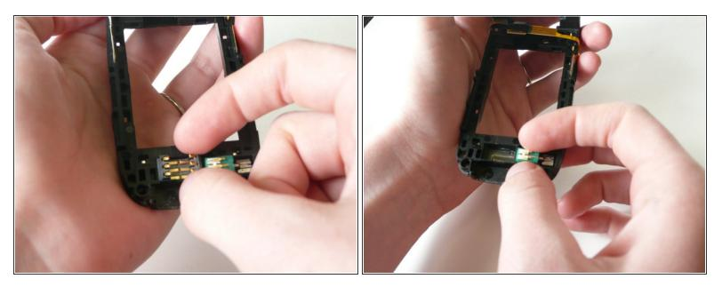
Remove the black sim card reader and green vibrator before continuing to ensure they do not fall out.
