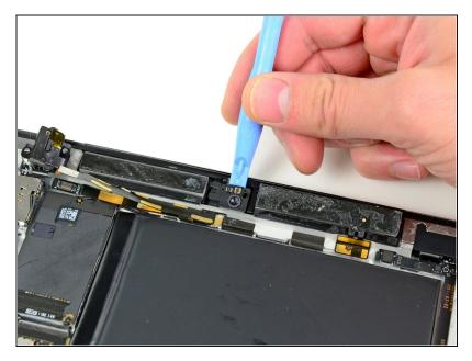
• Peel the front camera off the foam adhesive securing it to the rear panel.
