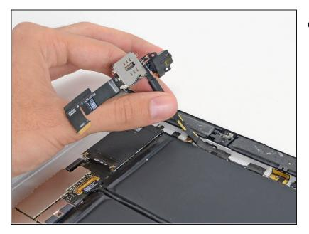
• Peel the front camera and microphone cables off the rear panel.
