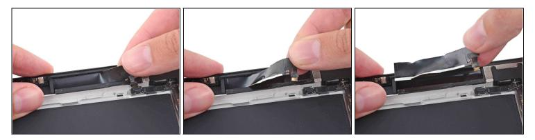
• As soon as you can grip the GPS antenna with your fingers, peel it up off the rear case to remove it.
