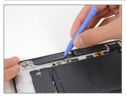
• Gently pry the cellular data antenna from the rear case with a plastic opening tool.
