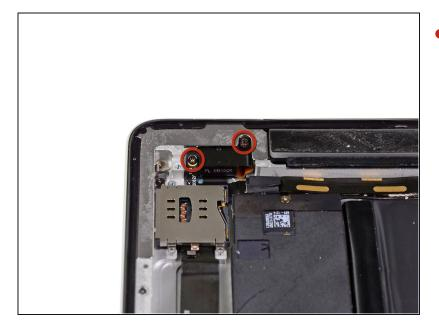
Remove the two 2.9 mm Phillips screws securing the headphone jack to the top edge of the rear panel.
