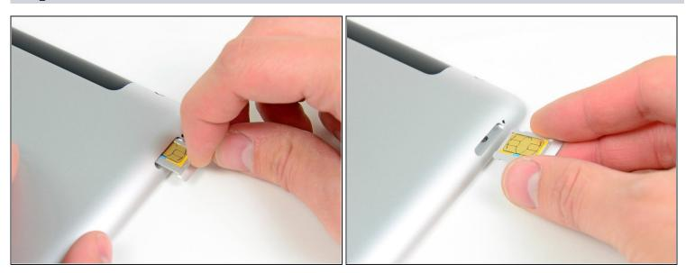
• Pull the SIM tray out of its slot and remove it from the iPad 2.
