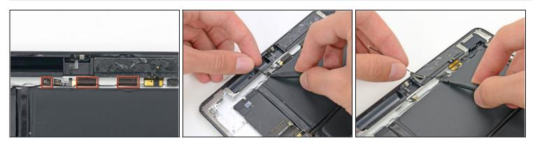
$\triangle$  In this step you will remove the three pieces of tape securing the right cell antenna cable to the rear case.
