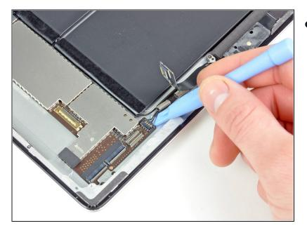
Place the prying tool beneath the 4 wires on the end of the connector and gently pry the speaker cable connector straight up from its socket on the logic board. <u>Do not pry</u> from the opposite end of the connector as this will break the 4 solder points on the underside of the socket and will require a microsolder repair.
