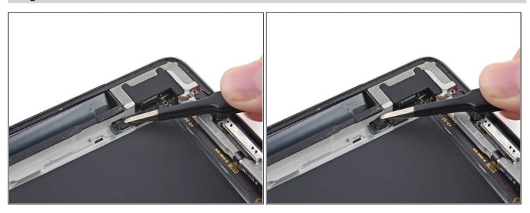
• Remove any tape covering the GPS antenna ZIF connector.
