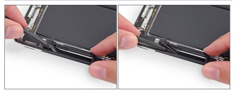
• Continue to push the spudger under the antenna to clear it of adhesive.
