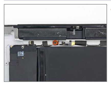
Remove the single 2.1 mm Phillips screw securing the cellular data antenna cable to the rear case.
