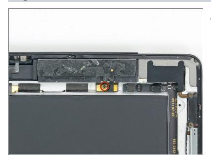
• Remove the single 2.1 mm Phillips screw securing the right cellular antenna to the rear case.
