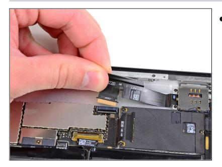
• Pull the headphone jack and front camera ribbon cable straight out of its socket on the logic board.
