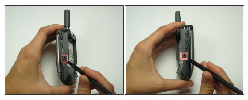
• Simultaneously press the highlighted buttons on both sides of phone.
