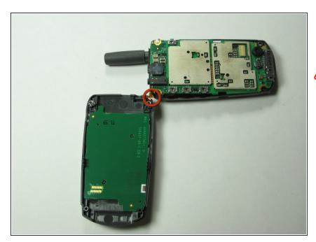
• Separate the back plate from the rest of phone.
