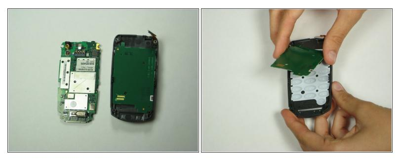
• Once logic board is removed lift the green keypad sensor for the front plate.
