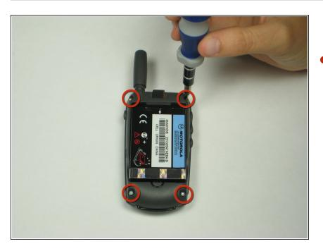
Using a T6 Torx screwdriver, remove the four screws from the back of the phone.
