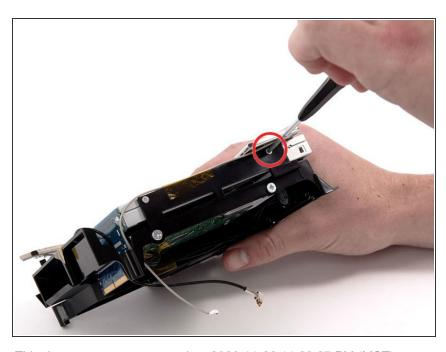
Remove the single silver Phillips screw from the black plastic framework directly below the Bluetooth antenna board.
