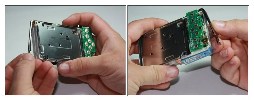
• Carefully pull off the side covers wrapped around the camera.
