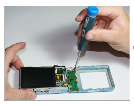
Using the Phillips #00 screwdriver, remove the eight black screws connecting the green keypad chip to the rear panel.
