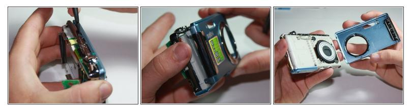
Using the spudger, gently lift off the front cover of the camera.
