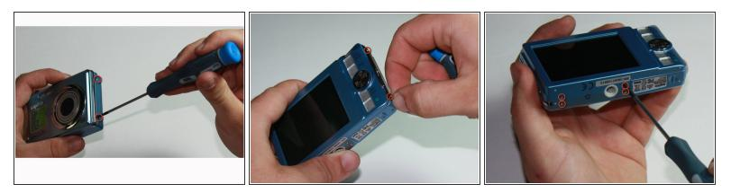
Remove the eight screws around the sides and bottom of the camera using a Phillips #00 screwdriver.
