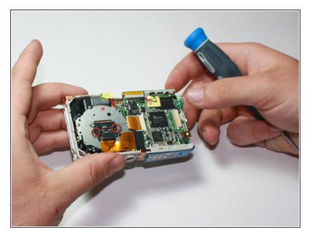
Remove the two screws holding the photo array.
