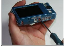
Remove the eight screws around the sides and bottom of the camera using a Phillips #00 screwdriver.
