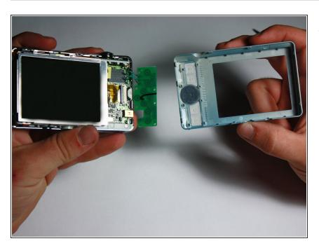
Separate the rear panel from the rest of the camera.
