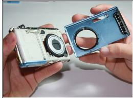
Using the spudger, gently lift off the front cover of the camera.
