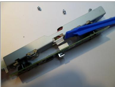
The connector of the mikrophone-array
