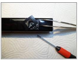
• The next two PH0 Screws are located BEHIND the two polycarbonate-plates of the two cameralenses. Take a sharp tweezer and stab under that plate. The plates are glued with a sticky tape to the housing. These plates are very fragile and will break if handled incautious.
