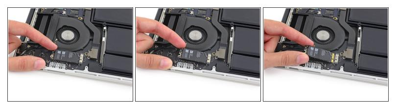
• Lift the free end of the AirPort board up slightly and pull it straight out of its socket on the logic board.
