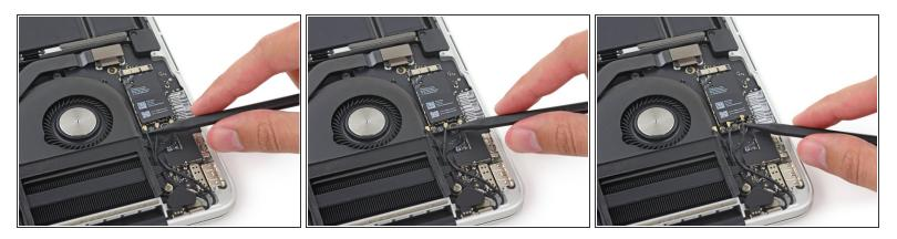
• Wedge the tip of a spudger underneath each of the antenna cables, near their connectors and pry up to disconnect them from the AirPort board.
