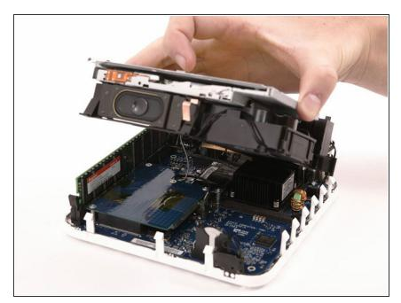
Grasp the optical drive and mass storage unit in one hand and lift up enough so that you can see beneath it.
