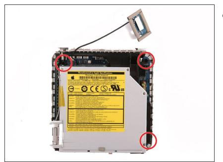
Remove the three black Phillips screws securing the plastic framework to the logic board and lower case.
