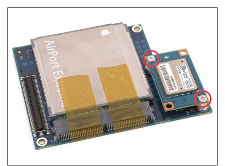
• Remove the two silver Phillips screws from the corners of the Bluetooth board.
