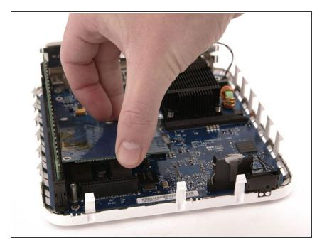
Grasp the board at the front and back, and lift up on the front until the board pulls free of its connector.
