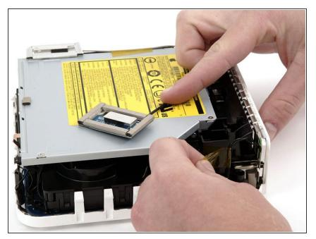
• Remove the yellow tape securing the power button cable to the black plastic framework.
