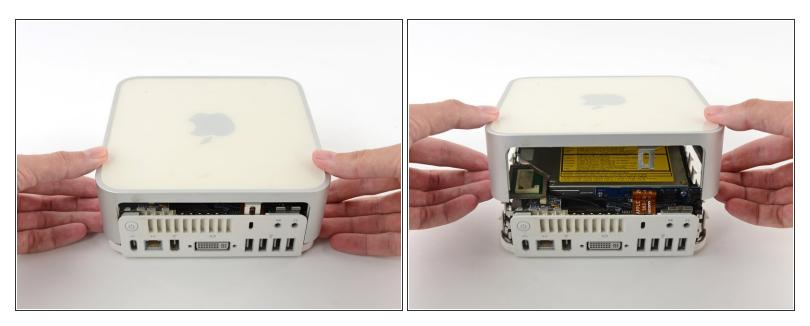
• Flip the Mac mini back over and lift the top housing off of the lower housing.
