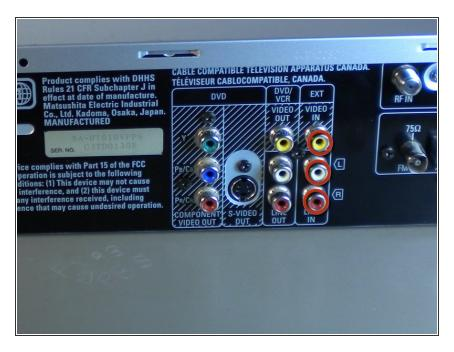
Make sure that cables going to the television are not connected to the outputs circled in red.
