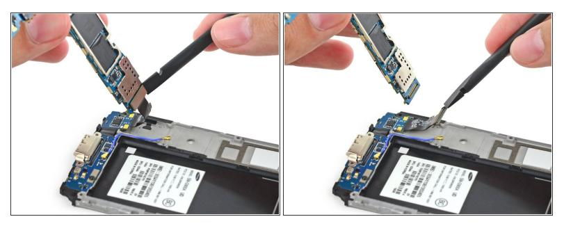
Use the flat end of a spudger to pry the daughterboard connector straight up off its socket on the motherboard.
