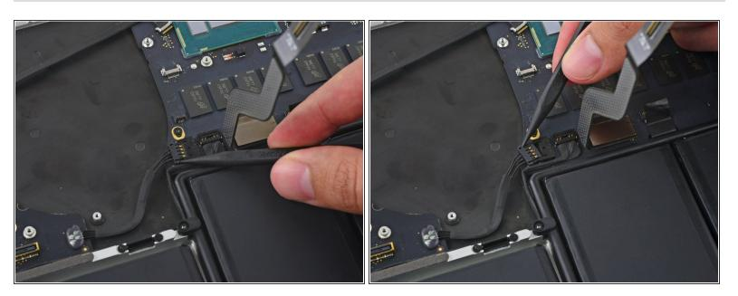
Use the tip of a spudger to push on either side of the I/O board connector to walk it out of its socket on the logic board.
