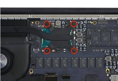
Use the flat end of a spudger to peel the four foam stickers off of the heat sink screws.
