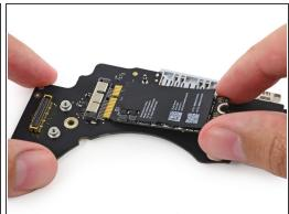
Lift the free end of the AirPort board up slightly and pull it straight out of its socket on the I/O board.
