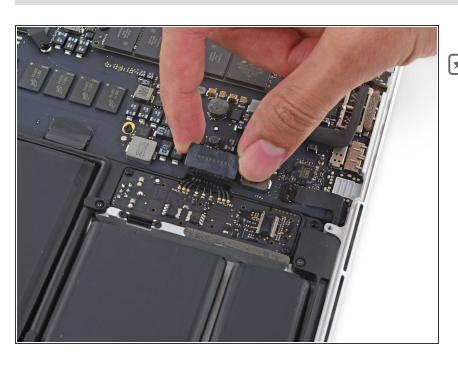
Bend the battery connector up out of the way to prevent accidental contact with its socket during your repair.
