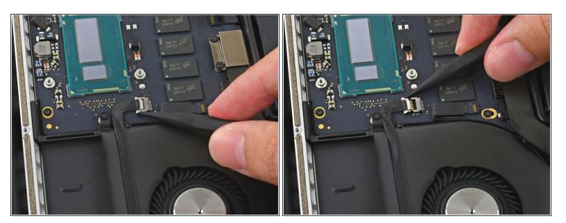
• Use the tip of a spudger to push on either side of the the iSight camera cable connector to walk it out of its socket on the logic board.
