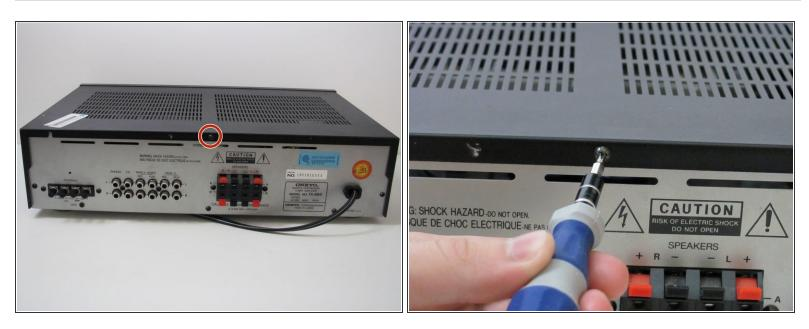
• Remove the top screw on the back panel.
