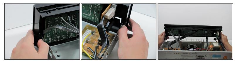
• Simultaneously push down on the head of the snap on each end of the device with your thumbs and push to seperate the face plate. This may take some force.
