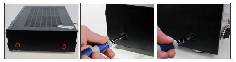
Remove the two screws on both sides of the receiver. Keep these and the rest of the screws in a safe place.
