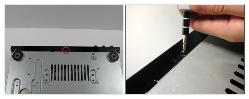
Unscrew the one screw on the bottom of the front panel.
