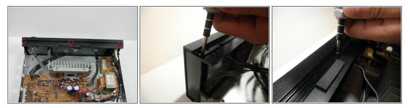
Unscrew the three screws on top of the face plate.
