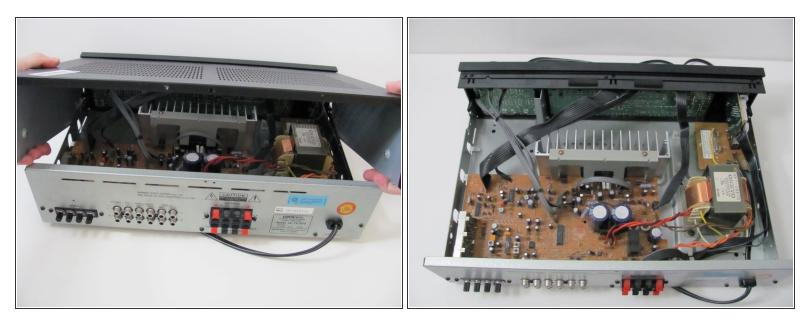
• Slide off the case to expose the internal components of the receiver.
