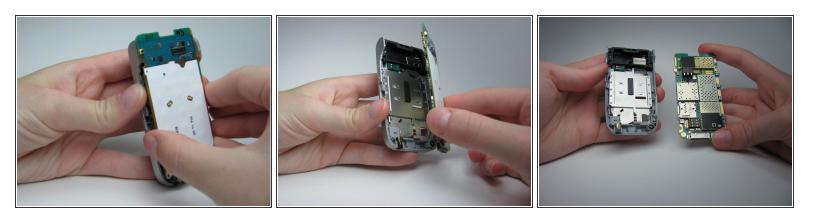
• Remove the logic board from the bottom casing.
