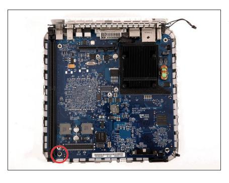
Remove the single black Phillips screw from the front left corner of the logic board.
