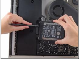
Use a spudger to disconnect the single SATA power and data combo cable.
