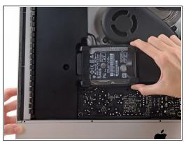
Lift the hard drive from the edge nearest the logic board and pull it slightly out of its recess.
