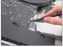
(i) If necessary, use the tip of a spudger to peel back the tabs covering the antenna connectors.
