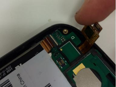
Next, use a platic spudger to remove the flex cable from its connection
