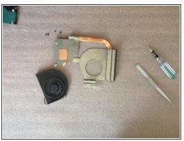
Disassemble the Heat Sink system to clean the fan and the radiator from inside.
