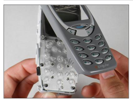
Remove keypad from under the face plate.
