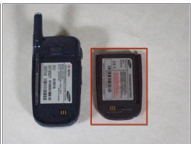
Push open the latch and remove the battery.
