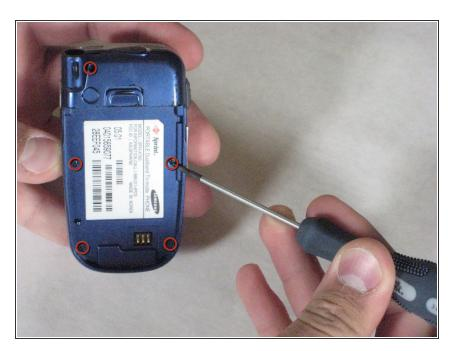
Remove the five screws as shown.
