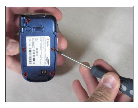
Remove the five screws as shown.
