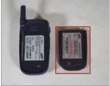
Push open the latch and remove the battery.
