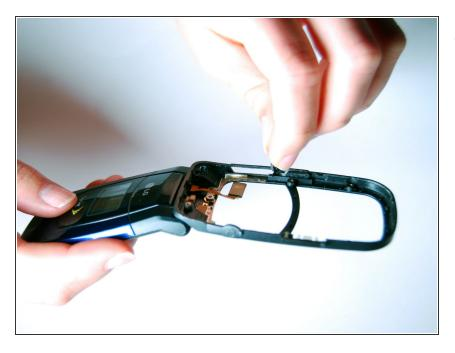
To finish the replacement, insert your new volume toggle button and reassemble your LG LX150 to resume use.
