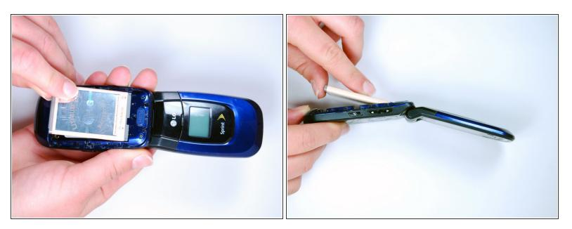
• Simultaneously push the battery forward and pull up from the bottom.
