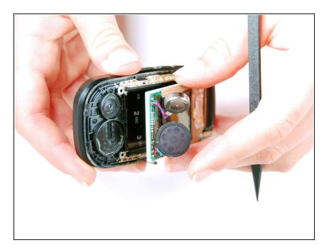
Using the spudger, pry between the speaker circuit board and base to detach with ease.
