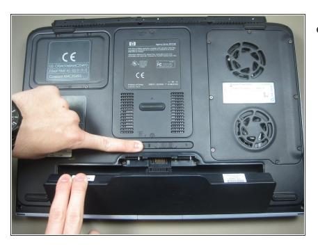
Slide the battery release switch to the right while simultaneously lifting up the battery.
