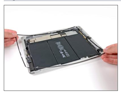
When the adhesive has been released along all the edges of the iPad, lift the plastic display bezel off of the iPad.
