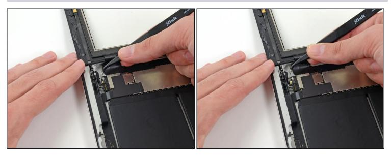
• Use a pair of <u>tweezers</u> to pull the home button ribbon cable straight out of its socket on the logic board.
