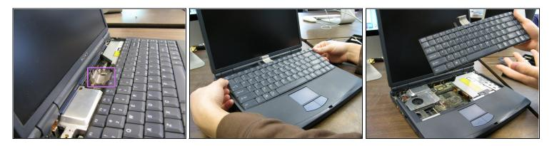
• To remove the keyboard, lift it a few inches from the computer, taking care not to pull beyond the length of the ribbon cable that secures it to the motherboard.
