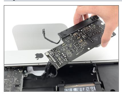
Remove the power supply from the iMac.
