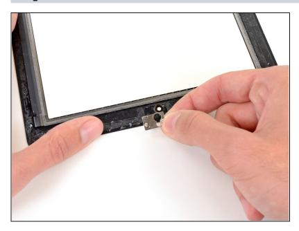
Lift and remove the camera bracket up off the front panel.
