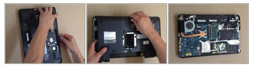
• With a plastic tool you can separate the bottom case from the laptop.
