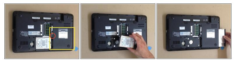
• Remove the HDD and the DVD optical drive.
