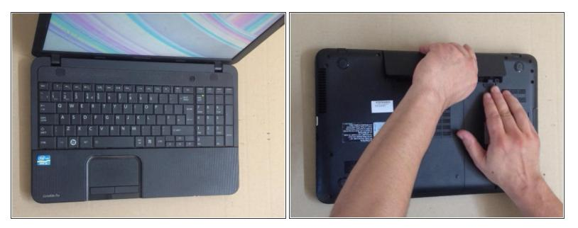
• Switch-off the laptop and remove the battery.
