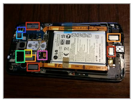
Now that the back case has been completely removed, it's time to disconnect all the ribbon cables connected to the two boards.
