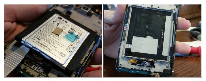
Now you need to get that battery out of there. I used a sturdier metal prying tool to CAREFULLY slide under the battery to free it from the adhesive. An old credit card might work better and pose less risk to the battery.
