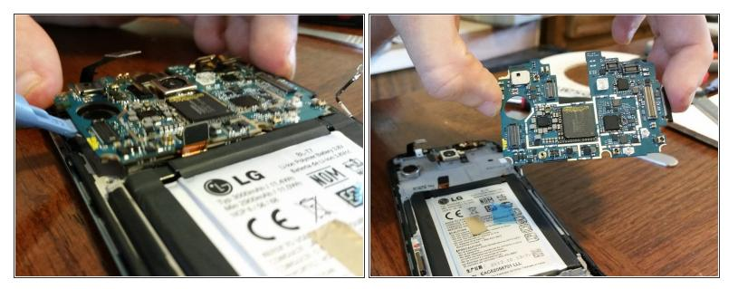
Make sure all of your ribbon cables are free of the board. Use your plastic prying tool and lift up on the board. If all of the cables are out of the way, it will come free.
