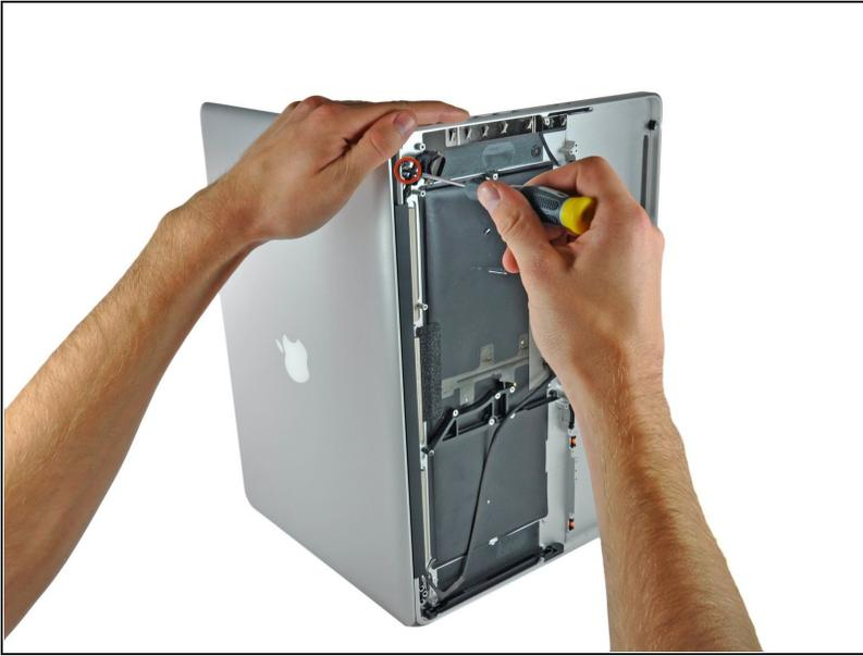
**⚠** Be sure to hold the display and upper case together with your other hand. Failure to do so may cause the freed display/upper case to fall, potentially damaging each component.
