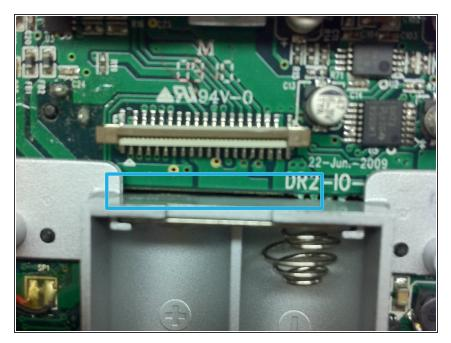
Feed the ribbon cable through this opening. This is much easier than disconnecting from the front circuit board, which requires delicate, if not impossible maneuvers to reconnect upon reassembly.
