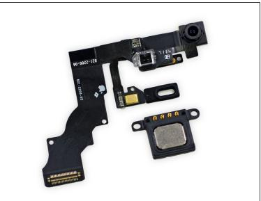
The front-facing camera is part of a larger cable assembly, which includes the earpiece speaker, microphone, and ambient light sensor. Both reside on the front panel assembly.
