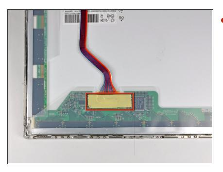
Remove the tape covering the display data cable on the LCD panel.
