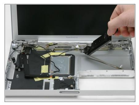
• Slide the subwoofer away from the screen and out of the computer.
