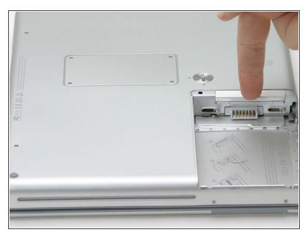
• Flip down the door on the right side of the battery compartment.
