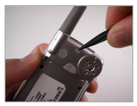
Remove the rubber grommet using a Spudger.
