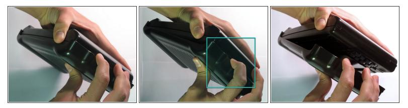
(i) The first step to any repair operation is to remove the front cover.
