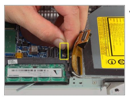
Disconnect the newly-revealed hard drive cable from the logic board.
