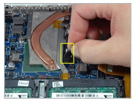
Peel up the small black rubber cover from the right side of the heat sink.
