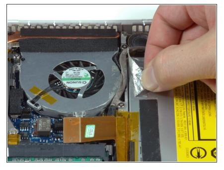
Peel up the foil tape between the fan and the optical drive.
