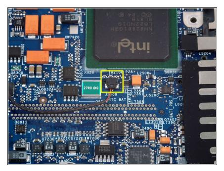
Disconnect the PRAM battery cable from the logic board and remove the PRAM battery from the computer.
