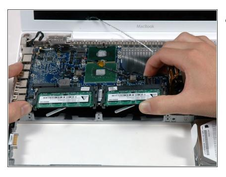
Lift the logic board up from the right side, and slide it up and out of the computer.
