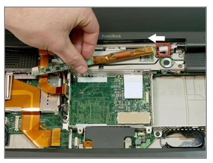
Disconnect the white inverter cable from the right end of the board
