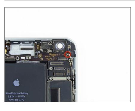
Remove the single 1.6 mm Phillips #00 screw securing the antenna clip to the rear case.
