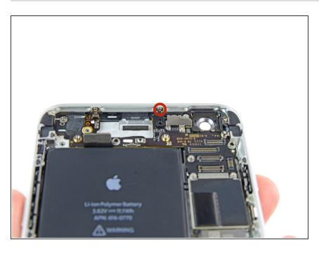
Remove the single 1.3 mm Phillips #00 screw recessed against the top of the rear case.
