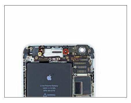
Remove the single 2.8 mm Phillips #00 screw securing the plastic clip to the logic board.
