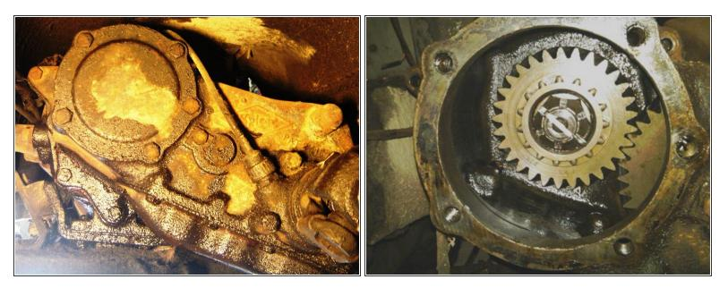
Next you'll need an impact gun or a large 1/2 inch drive breaker bar to remove the nut from inside the transfer case. It is behind the round cover on the transfer case. You should also remove the speedometer cable from the transfer case. This would be a good time to disconnect the drivelines, wrap tape around the U-joints to keep the caps from falling off and losing the needle bearings. I use pieces of coat hanger to hang the drive lines.
