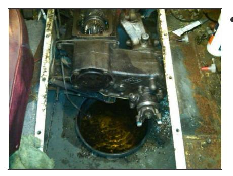
• To drain the fluid there are drain plugs on the transmission and transfer case, I still had quite a bit of oil in my transmission so you may get a mess when separating the units. There is a bolt that goes in from the front of the transmission into the transfer case, just to passenger side be sure to remove it. The two may be removed as a single unit but it's harder to maneuver it out of the hole and much heavier. ( or if you have the equipment you can drop it under after removing the shifters)
