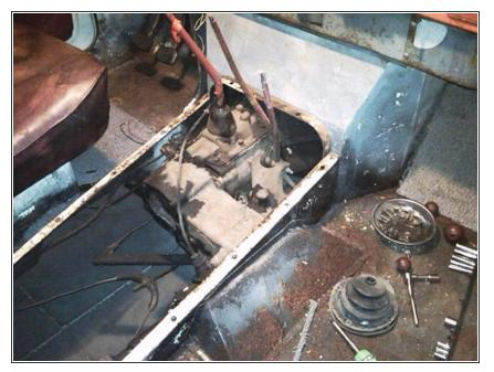
Start with removing passenger seat. Remove shifter boots and shift knobs. Next the center transmission/transfer case cover inside the vehicle.
