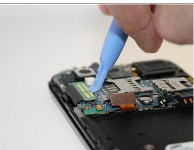
Use the plastic opening tool to detach the two tabs connecting the motherboard to the base of the phone.
