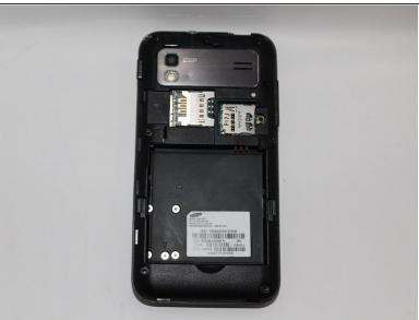
Remove the seven screws from backplate using the #00 screwdriver.
