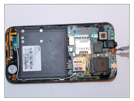
Remove the single screw connecting the motherboard to the base of the phone by using the #00 Phillips screwdriver.
