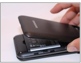
Remove back cover using fingernail or plastic opening tool. The cover pulls up and off.
