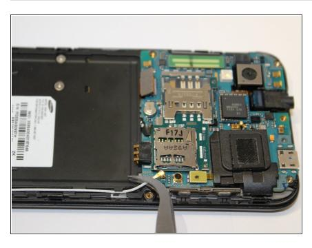
Disconnect the antenna cable from the motherboard using tweezers.
