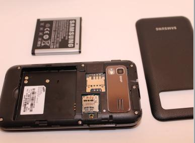
Remove battery with plastic opening tool or finger.
