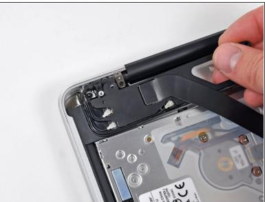
Before securing the AirPort/Bluetooth bracket to the upper case, be sure the small plastic tab on its left edge is inserted into the small void cut into the black plastic optical drive opening.
