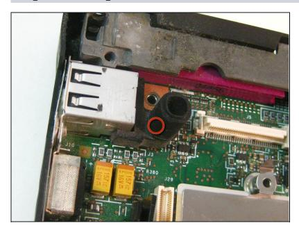
Remove the rubber cover from the microphone.
