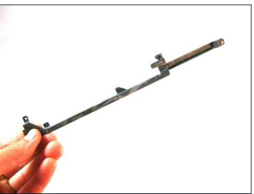
• Grasp the metal bracket to remove it from the device.
