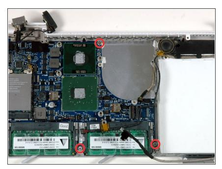
Remove the three Phillips screws securing the logic board to the lower case.
