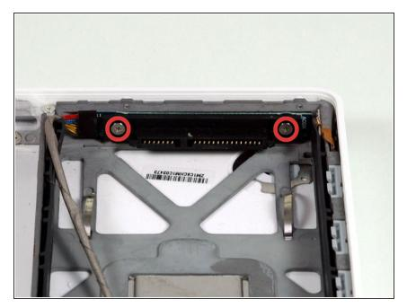
Remove the two Phillips screws securing the hard drive connector to the lower case.
