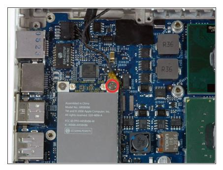
Remove the single Phillips screw in the upper right corner of the Airport card.
