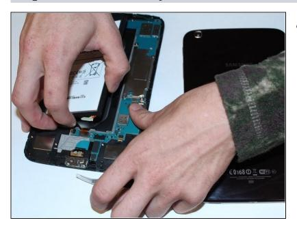
After the battery is disconnected, use the pulling tab to safely remove the battery.
