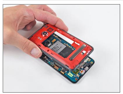
• Remove the rear inner frame from the rest of the Evo.
